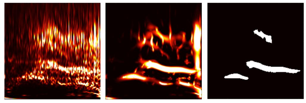
Suppression: TF plot is smoothed using the guided filter and a bounded thresholding is applied for extracting the suppression mask
