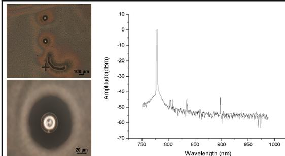
The devices pictured above have been coated with liquid silica containing a  $Ti(OBu)_4$  to MTES molar ratio of 0.05 and 5 wt% Nd. Lasing spectra demonstrates Cascaded Raman lasing, but no Nd lasing. Raman lasing was observed at input powers above 1 mW, suggesting two major implications:
