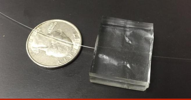
We have demonstrated that our fiber-based polarimetric stress sensor can measure the Young's modulus of materials with different stiffnesses. The next step is to prepare the testing setup to accommodate tissue samples and to measure the Young's modulus of various real tissue samples. Based on these preliminary results, we believe our sensor will be able to distinguish between materials with different stiffness and will be a valuable tool for diagnostic researchers.
