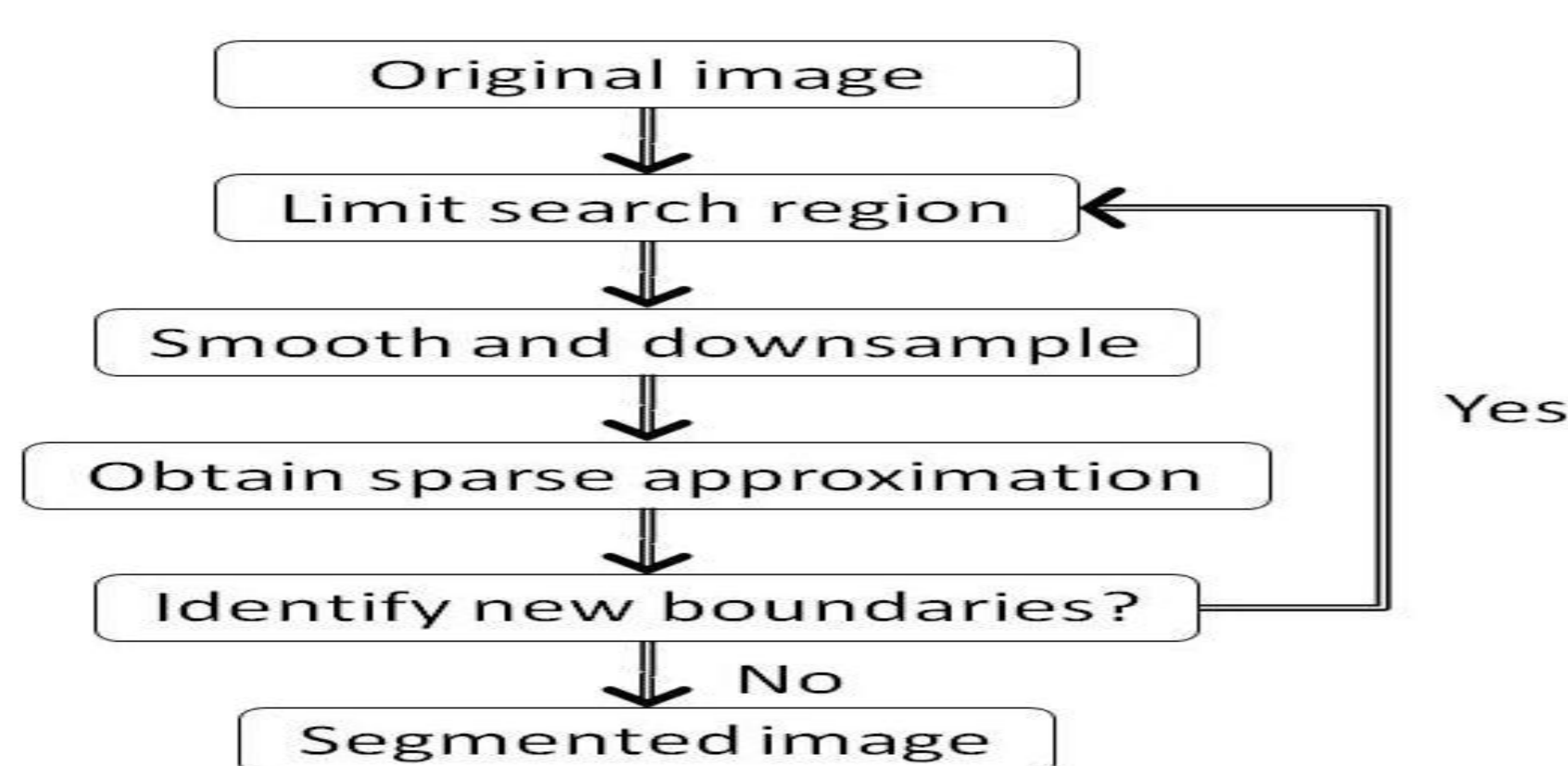
Figure 2: Schematic of layer segmentation algorithm
