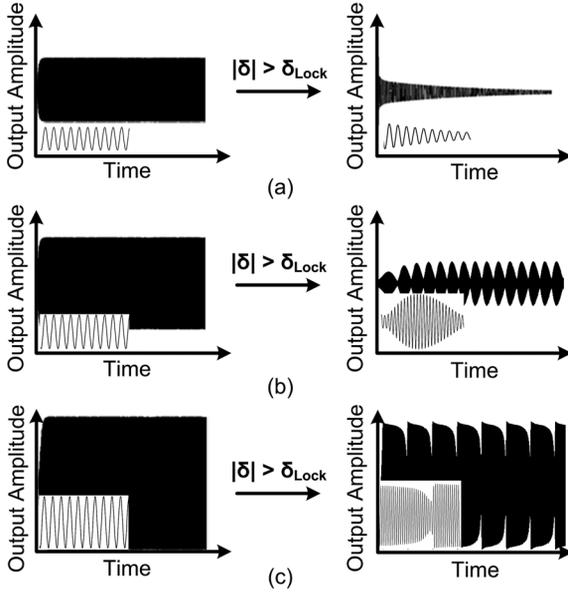
Fig. 11. Different scenarios for the oscillator output signal, when it is detuned more than it can tolerate at different  $V_{in}$ : (a)  $V_{in1}$ , (b)  $V_{in2}$ , and (c)  $V_{in3}$ , where  $V_{in1} < V_{in2} < V_{in3}$ . Zoomed versions are shown in the respective insets.
