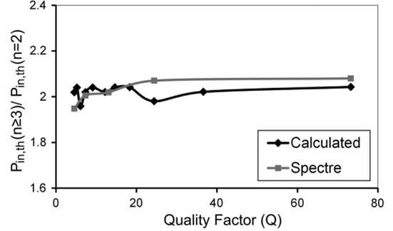
Fig. 7. Normalized minimum required input power for startup  $P_{in,th}(n \geq 3)/P_{in,th}(n = 2)$  versus resonator quality factor ( $Q$ ).
