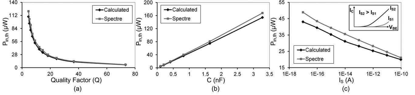
Fig. 5. Minimum required input power for startup  $P_{in,th}$  when  $n = \omega_{in}/\omega_{out} = 2$  versus: (a) resonator quality factor  $Q$ , (b) resonator capacitance  $C$ , and (c) BJT saturation current  $I_S$ .
