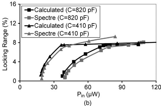
Fig. 14. Locking (tuning) range versus input power at  $N = 2$  for: (a)  $Q = 13$  and 6 and (b)  $C = 820$  pF and 410 pF.
