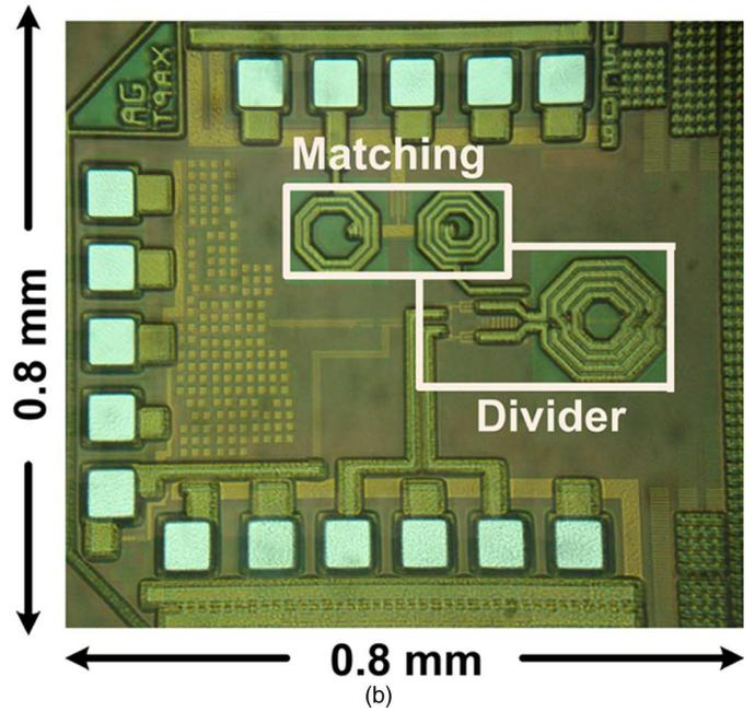
Fig. 21. (a) Detailed schematic and (b) chip microphotograph of the integrated 12-GHz divide-by-2 self-powered divider.
