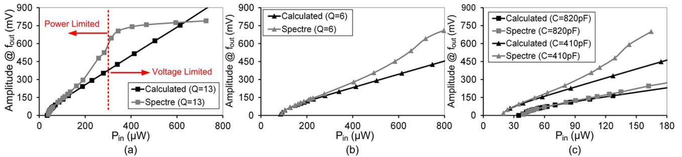
Fig. 8. Variation of the steady-state amplitudes  $r_{ss}$  as  $P_{in}$  varies for  $f_{in} = 2f_{out} = 5.29$  MHz when: (a)  $Q = 13$ , (b)  $Q = 6$ , and (c)  $C = 810$  pF and 410 pF.
