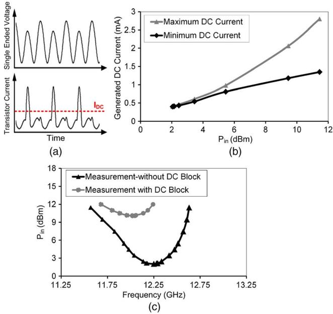
Fig. 24. (a) Simulated single-ended voltage and transistor current waveforms. (b) Measured maximum/minimum generated dc current in the 12-GHz divider. (c) Measured sensitivity curve with/without dc block at the input.
