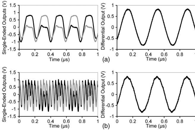
Fig. 18. Measured single-ended and differential output waveforms when: (a)  $f_{in} = 2f_{out}$  and (b)  $f_{in} = 10f_{out}$ .
