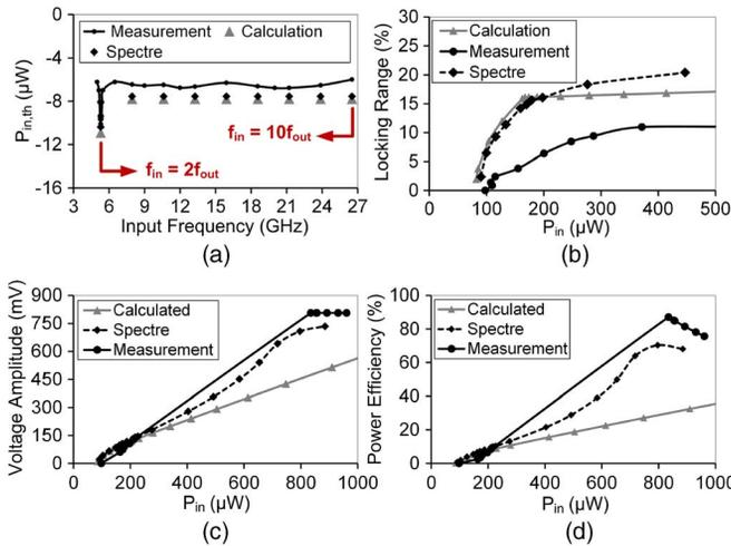
Fig. 19. Measured, simulated, and calculated: (a) minimum required input power ( $P_{in,th}$ ) for subharmonic generation versus the input frequency, (b) locking (tuning) range, (c) output amplitude, and (d) power efficiency versus input power at  $n = 2$ .
