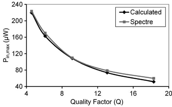
Fig. 13. Input power at the edge of oscillation dying and pulling versus tank quality factor (Q).
