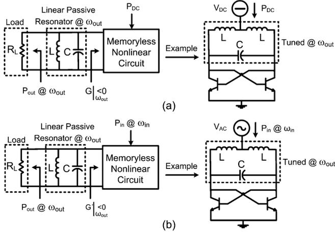
Fig. 1. (a) Negative resistance oscillator. (b) Proposed passive subharmonic generator using memoryless nonlinearity.
