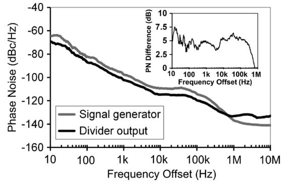
Fig. 23. Measured phase noise of the signal generator and the 12-GHz divider output.
