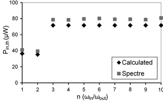
Fig. 6. Minimum required input power for startup  $P_{in,th}$  versus  $n = \omega_{in}/\omega_{out}$  when  $Q = 13$ .
