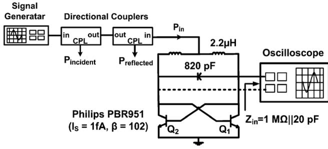
Fig. 17. Measurement setup for the low-frequency prototype.
