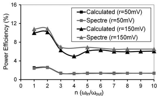
Fig. 10. Variation of the power efficiency  $\eta$  versus  $n$  for  $r = 50$  mV and  $r = 150$  mV when  $Q = 13$ .
