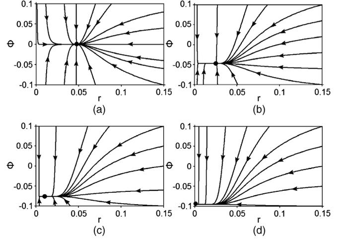
Fig. 12. Phase portrait of the circuitry around the stable point at different values of  $n$ : (a)  $n = 2$ , (b)  $n = 1.97$ , (c)  $n = 1.95$ , and (d)  $n = 1.93$  for  $Q = 13$  and  $V_{in} = 0.695$  mV.
