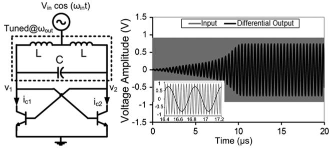
Fig. 2. Input/output voltage waveforms when  $f_{in} = 26.4$  MHz and  $f_{out} = 2.64$  MHz ( $f_{in} = 10f_{out}$ );  $L = 2.2$   $\mu$ H,  $Q = 13$ , and  $C = 820$  pF. A zoomed version is shown in the inset.
