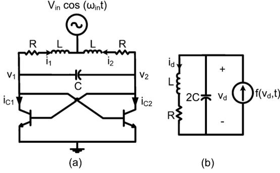
Fig. 3. (a) Self-powered downconverter with state-variables. (b) Second-order model for the downconverter.
