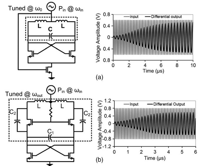
Fig. 25. Alternative configuration for the proposed passive subharmonic generator without any dc power supply and their representative input/output waveforms. (a) Differential cross-coupled oscillator with tail transistor ( $f_{in} = 2f_{out} = 5.29$  MHz). (b) Differential noise-shifting Colpitts oscillator ( $f_{in} = 2f_{out} = 9$  MHz) [25].
