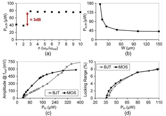
Fig. 16. Simulated minimum required input power for startup  $P_{in,th}$  versus: (a)  $n = \omega_{in}/\omega_{out}$  and (b) nMOS channel width  $W$  at  $n = 2$ ; (c) the steady-state amplitudes  $r_{ss}$ , and (d) locking (tuning) range versus  $P_{in}$  at  $n = 2$  and  $Q = 13$ .
