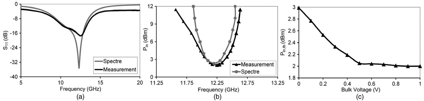
Fig. 22. Measured and simulated: (a)  $S_{11}$  (return loss), (b) sensitivity curve, and (c) measured  $P_{in,th}$  versus the transistor bulk voltage.
