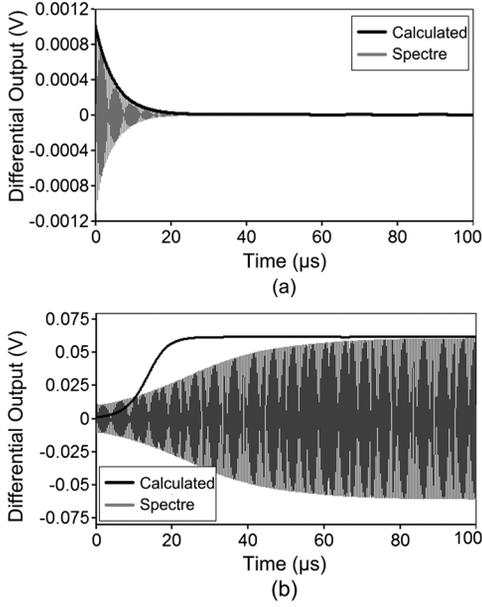
Fig. 4. Transient behavior of the circuitry for: (a)  $V_{in} = 0.68$  V and (b)  $V_{in} = 0.7$  V.
