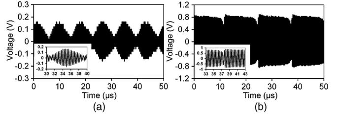
Fig. 20. Measured output waveforms when the downconverter is pulled for  $n = 2$  at: (a)  $P_{in1}$  and (b)  $P_{in2}$ , where  $P_{in1} < P_{in2}$ . Zoomed versions are shown in the respective insets.
