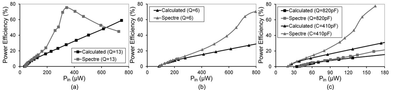
Fig. 9. Variation of the power efficiency  $\eta$  as  $P_{in}$  varies for  $f_{in} = 2f_{out} = 5.29$  MHz when: (a)  $Q = 13$ , (b)  $Q = 6$ , and (c)  $C = 810$  pF and 410 pF.
