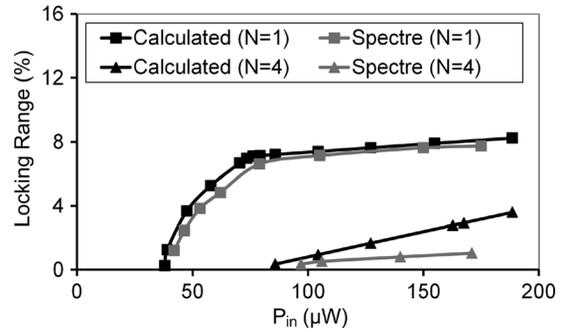
Fig. 15. Locking (tuning) range versus input power at  $N = 1$  and  $N = 4$  for  $Q = 13$ .
