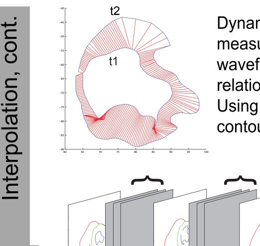
Dynamic time warping works by measuring "similarity" between waveforms t1 and t2 and draws relationship lines between similar points. Using these lines new intermediate contours can be drawn along those lines.
