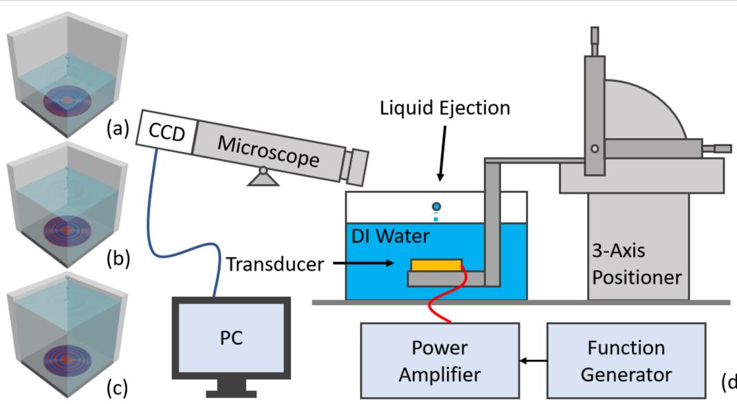
(a)-(c) Schematics illustrating that water droplets can be ejected at different water height due to the transducer's tunable focal length. (d) Measurement setup to observe droplet ejection with a CCD camera, while the focal length is measured with a micro-positioner.
