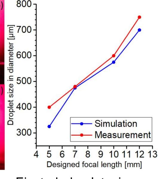
Ejected droplet size vs designed focal length (both measured and simulated data).
