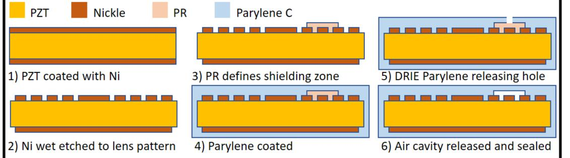
Brief microfabrication process of the transducer.
