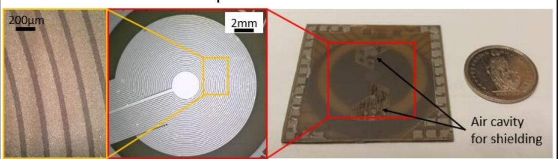
Fabricated device with air cavity blocking acoustic wave.
