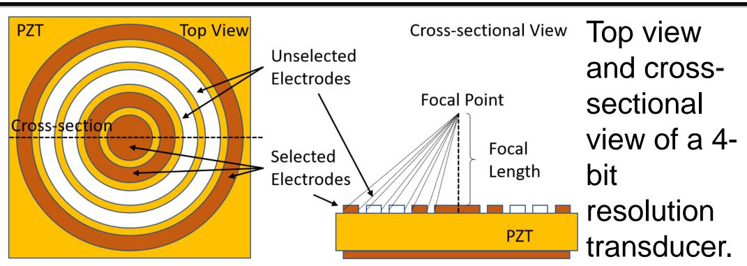
Each of the four equal-width concentric ring electrodes can be selected to generate ultrasound. By varying the selection, the focal length can be varied.
