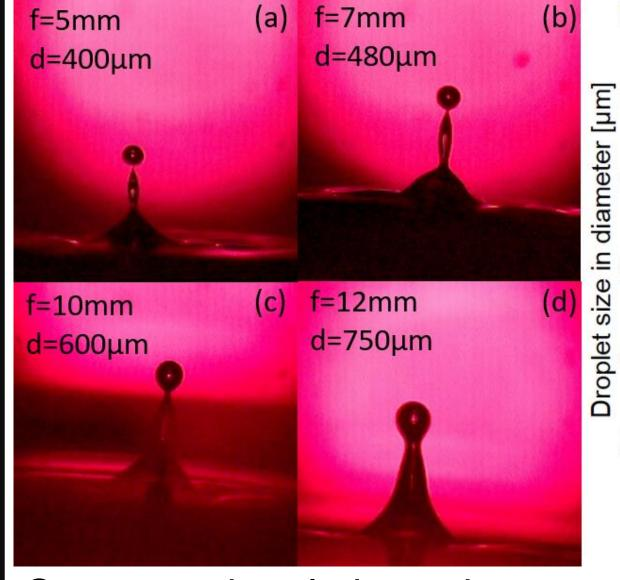
Cross-sectional-view photos of droplet ejections obtained at the water heights of 5mm (a), 7mm (b), 10mm (c), and 12mm (d).
