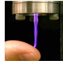
Transient (“cold” plasma) produced by nanosecond pulses
