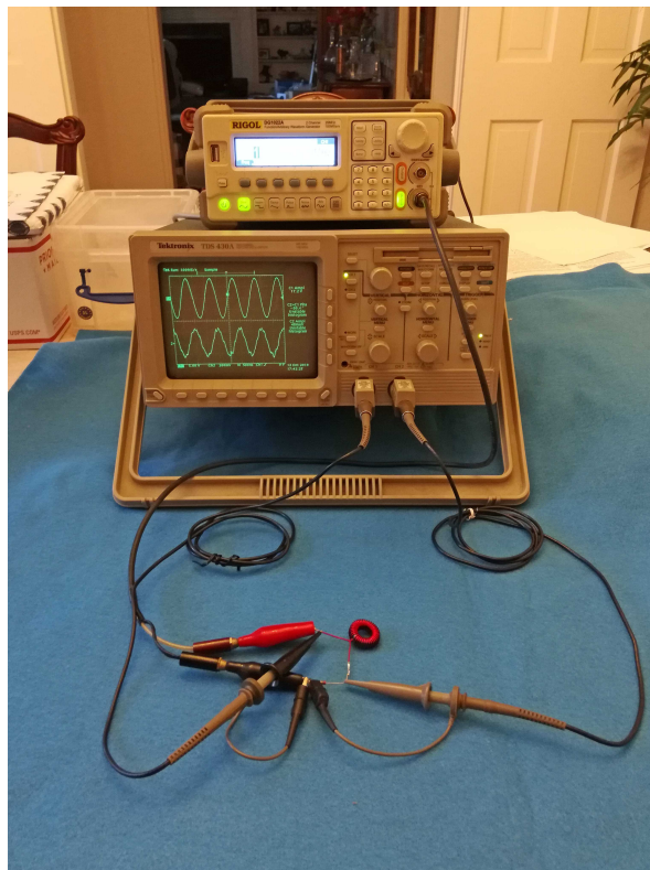
Figure 9: Faraday's law circuit connected to instrumentation.
