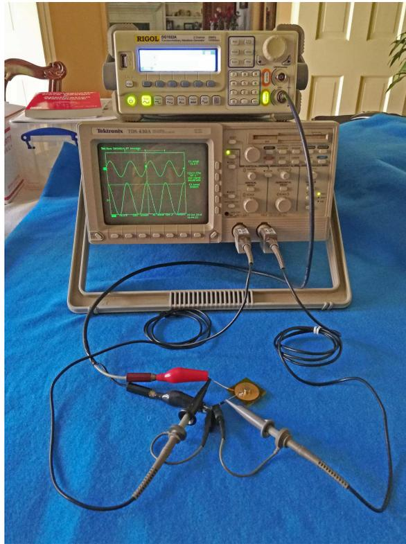
Figure 7: Ampere's law circuit connected to instrumentation.
