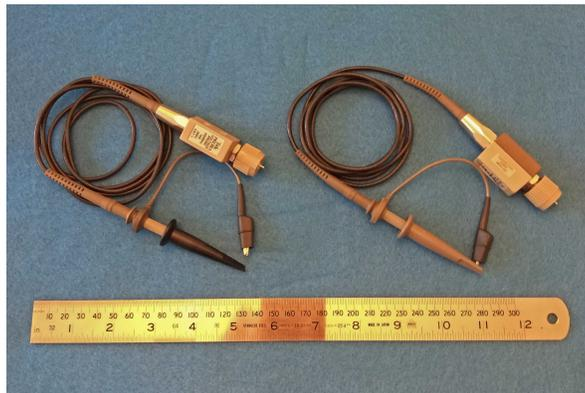
Figure 6: Oscilloscope probes.
